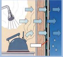
We put over 1,000 vapor holes\* in every square foot of WeatherAll®. These tiny holes enhance water vapor permeability. This important feature helps ensure that water vapor can escape the wall cavity. Trapped water vapor can cause mold formation and, if unnoticed, can lead to structural damage.
