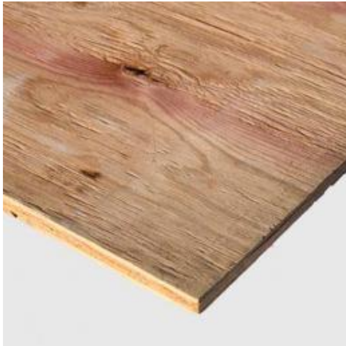
15/32" 48"X96" Rated Sheathing Exposure 1 Western 5PLY 32/16
